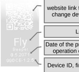
website link to manage and change device settings Logo Date of the prepaid period of operation of the device Device ID, firmvare version
