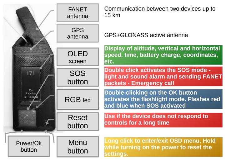
Power on/off — press and hold until the screen turns on/off. Double click activates flashlight. On OSD menu activates/changes properties.
